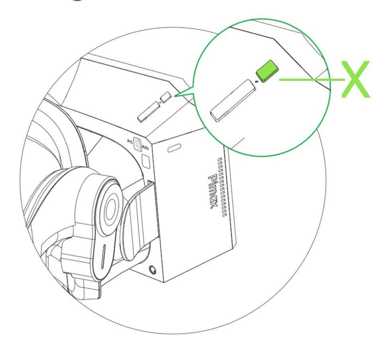
7. Connect the DP cable to your headset You should hear a clicking sound to confirm that it has been properly connected.
